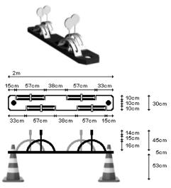
The point at which the target disc is attached to the pivot arm and the pivot mechanism at the bottom of the arm are subject to very high impact forces and must be strong and well constructed.
